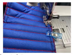
24. Join the side panels at the center bottom.
