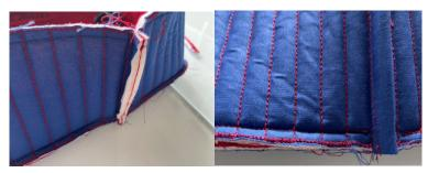
26. Bind the edges of the seam you just made. Repeat with the front part of the backpack. It may be necessary to make some small tucks in the rounded edges, but that is ok.
